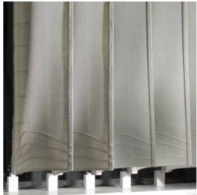
Fig.9: Laminate with reinforcements, accordingly placed to the tensile stress lines and leaf venation pattern.
