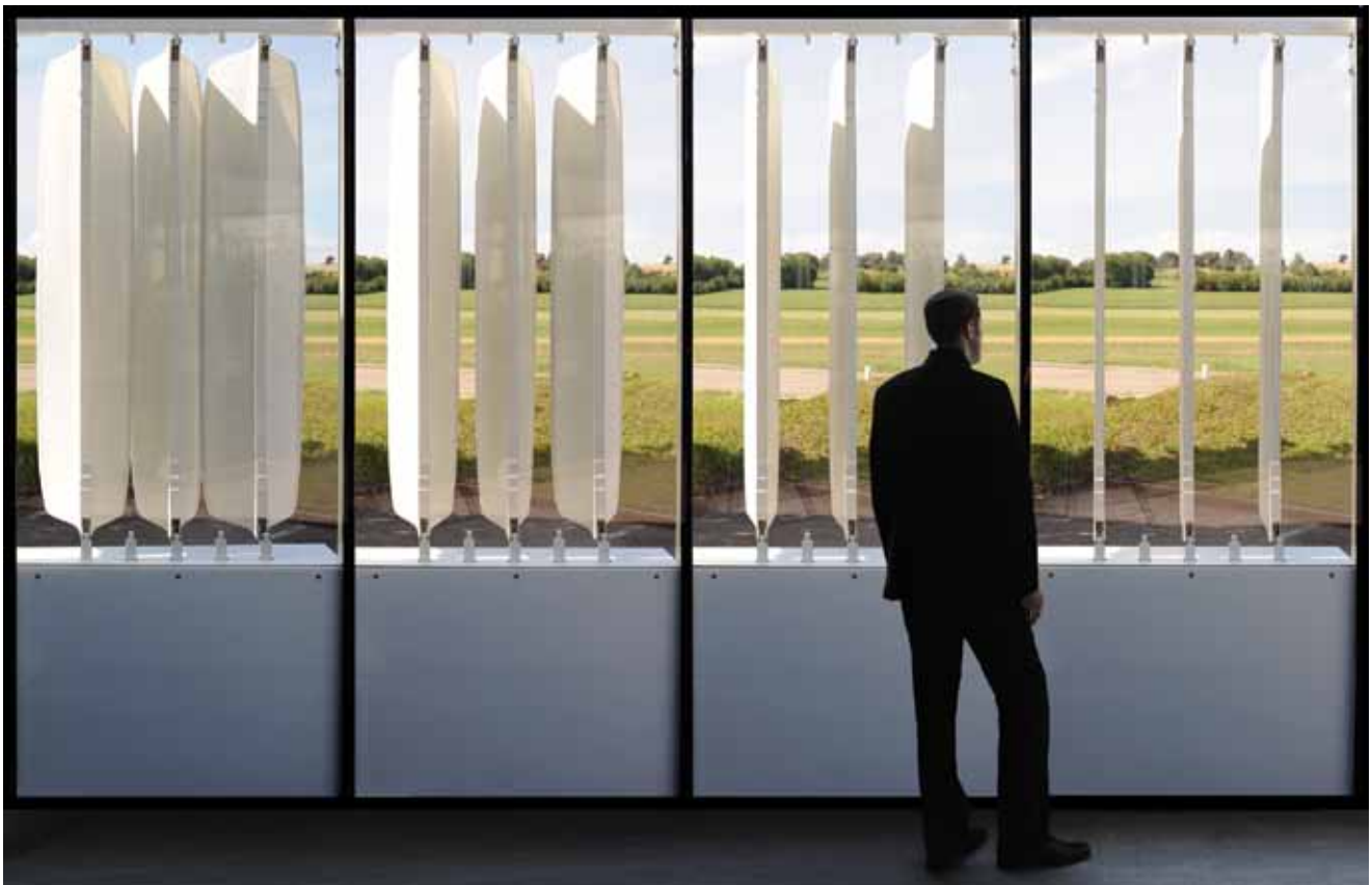
Fig.7: Full-scale prototype of the Flectofin® Facade, produced with the industrial partner clauss markisen. The lower support of the GFRP lamellas can be moved vertically and thus cause the eccentrically attached backbone to bend.
